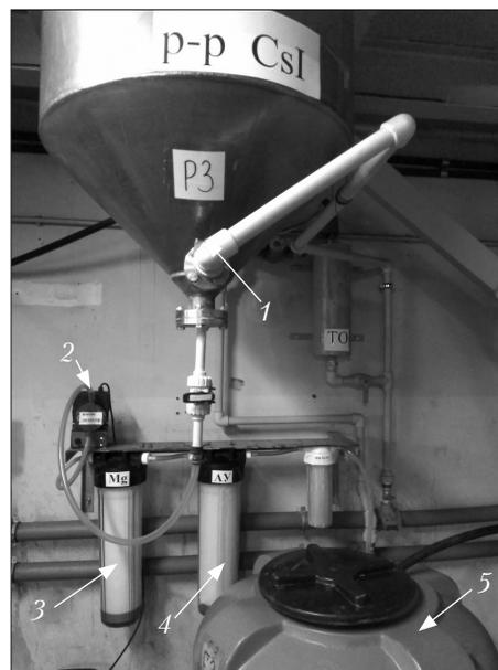
**Fig. 2.** The view of the experimental-industrial node of CsI purification by filtration through cartridge filters filled with magnesium and carbon: 1 – heat-exchange apparatus (titanium); 2 – metering pump; 3 – Mg-filled cartridge filter; 4 – activated carbon-filled cartridge filter; 5 – capacity for the filtered solution
