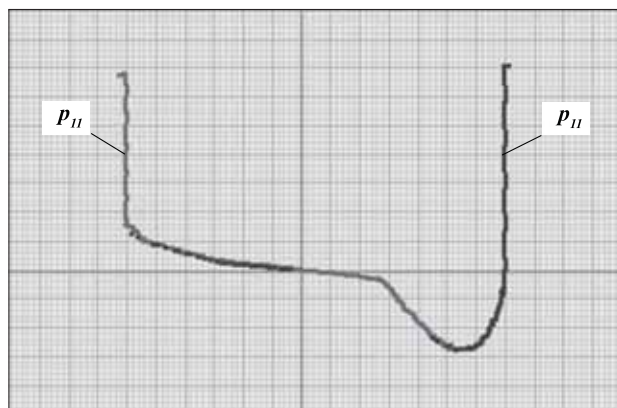
Fig. 5. General metric profile describing the wheel effective part
