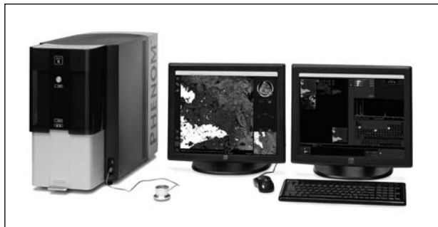
Fig. 1. External view of Phenom ProX desktop electronic microscope
