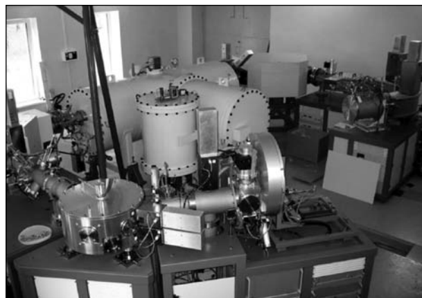
Fig. 1. AMS Tandetron 1.0 MV, model 4110Bo-AMS
