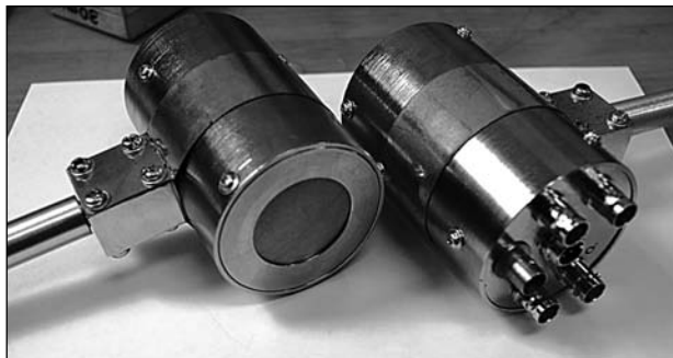
Fig. 5. External view of input block of ionizing radiation detector with entrance protective window
