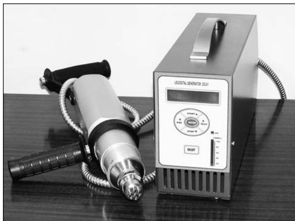
Fig. 2. Digital ultrasonic generator with vibro-impact tool
