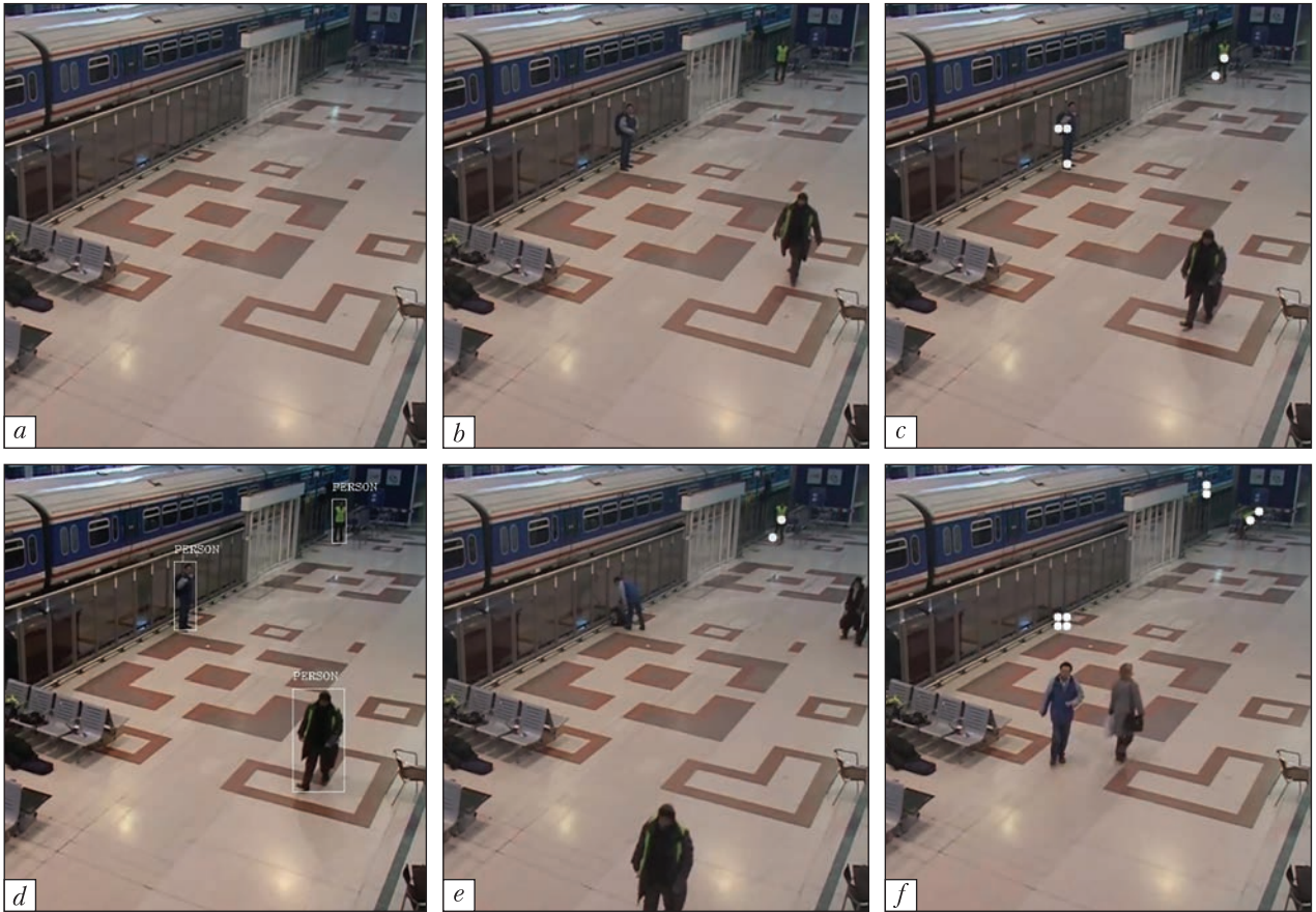
Fig. 2. Image from a video fragment illustrating a train station scenario: a – background image; b – a person has appeared but has not yet been marked as an abandoned object; c – the person has remained stationary and is marked as an abandoned object; d – recognition procedure performed, the object was identified as a person, the mark was removed; e – newly marked objects; f – objects with removed and retained markings
