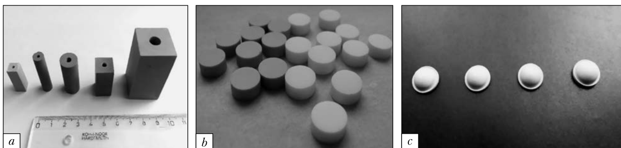
Fig. 2. High-quality dielectric resonators: a – coaxial for the decimeter range; b – “open” for the centimeter frequency range at H_{018} type of oscillations; c – in the form of a hemisphere
