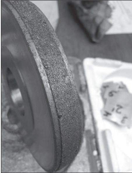
Fig. 7. Working surface of the diamond truing roller in a plan view: the middle part with CVD-diamonds and the two outer sections with HPHT-diamonds (grains of powder AC200T 400/315 evenly distributed) are depressed, as the baseline
