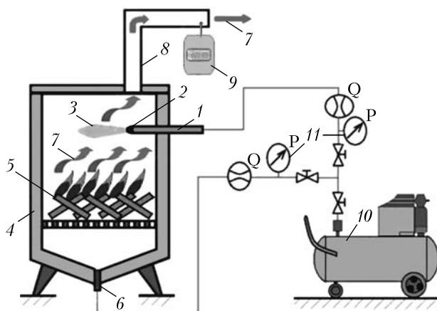
**Fig. 3.** Functional scheme of the physical model for the study of the postcombustion of outlet gases containing CO: 1 – lance; 2 – experimental nozzle; 3 – blowing gas jet; 4 – working unit; 5 – burning fuel; 6 – bottom nozzle for sustaining combustion; 7 – output gases that contain CO; 8 – metal pipe; 9 – CO measurement sensor Air quality detector E18609; 10 – air compressor; 11 – manometers
