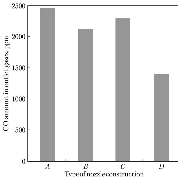
**Fig. 7.** The amount of CO in the outlet gases for the blowing through comparative nozzle (A) and coherent-type nozzle with a different ratio of the peripheral part to the total area of the nozzle (B – 25%; C – 50%; D – 75%)
