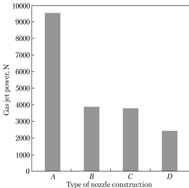
**Fig. 4.** Comparison of the jet power under the conditions of a flow rate of 2M flowing through comparative nozzle (A) and coherent-type nozzle with a different ratio of the peripheral part to the total area of the nozzle (B – 25%; C – 50%; D – 75%)
