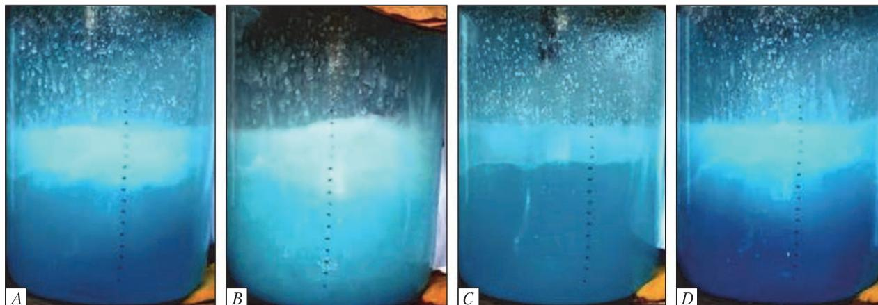
**Fig. 5.** Comparison of the results of blowing of two phase cold model through comparative nozzle (A) and coherent-type nozzle with a different ratio of the peripheral part to the total area of the nozzle (B – 25%; C – 50%; D – 75%)
