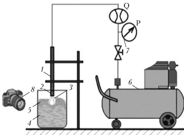
**Fig. 2.** Functional scheme of the cold two-phase simulation stand: 1 – top lance; 2 – experimental nozzle; 3 – gas jets; 4 – water; 5 – silicone oil; 6 – air compressor; 7 – manometer; 8 – camera
