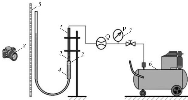
**Fig. 1.** Scheme of the experimental setup for the study of the force effect of the jet flowing out of nozzles of various configuration: 1 – top lance; 2 – experimental nozzle; 3 – gas jet; 4 – U-tube manometer installation; 5 – ruler; 6 – air compressor; 7 – manometers; 8 – camera
