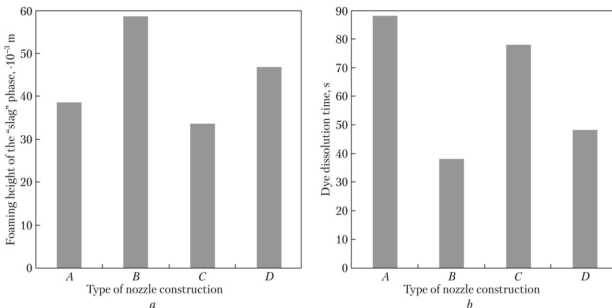
**Fig. 6.** The results of measuring foaming height of the second – “slag” phase (a) and the dissolution time of the dye (b) when blowing through a comparative nozzle (A) and a coherent type nozzle with a different ratio of the peripheral part to the total area of the nozzle (B – 25%; C – 50%; D – 75%)
