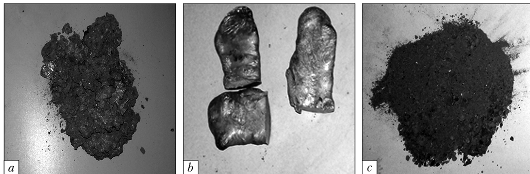
Fig. 1. General appearance of raw materials (a), samples of aluminum (b) and slag obtained after melting (c)
