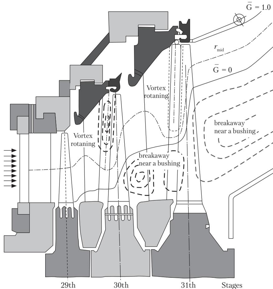
**Fig. 2.** Areas of vortex flows in the flow path of cogeneration turbine low-pressure cylinder at low-flow rate modes
