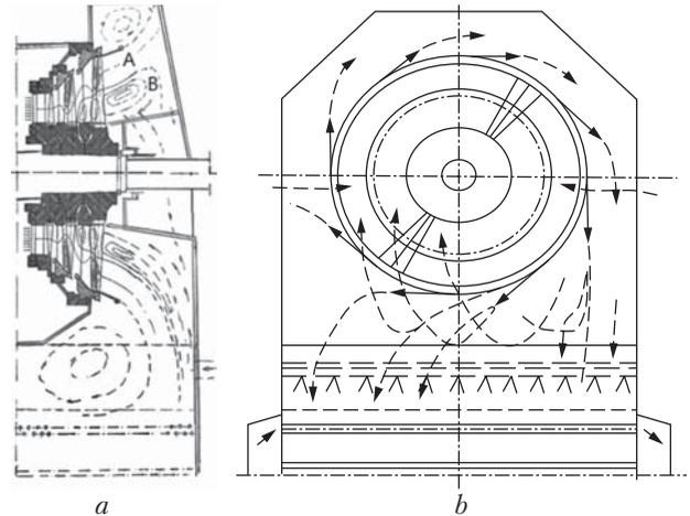
**Fig. 1.** Structure of the flow behind the working wheel of the last stage with a large fanning: *a* – longitudinal section; *b* – cross section; *A* – main flow; *B* – breakaway near a bushing
