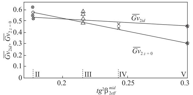
Fig. 6. Dependence of relative volumetric flow values on  $\text{tg}^2 \beta_{2eff}^{mid}$  (at  $\gamma_m = 0^\circ$ ): II–V are experimental model stages [8]
