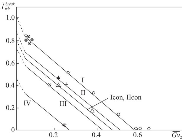
**Fig. 3.** Formation of the breakaway near a bushing depending on the height of the working blade and the volumetric steam flow: I–IV are experimental model stages [8]; Icon, IIcon are stages with a conical meridian bypass in the guiding apparatus
