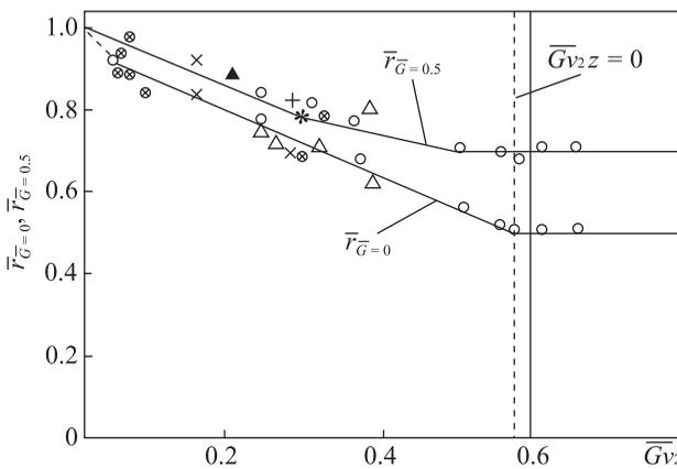
**Fig. 4.** Change in the position on the point attachment radius of the line  $\bar{G} = 0$  and  $\bar{G} = 0.5$  to working blades trailing edges
