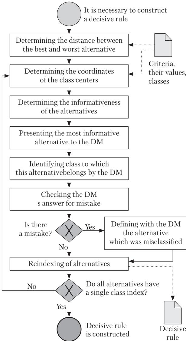
Fig. 1. Procedure for constructing a decisive rule
