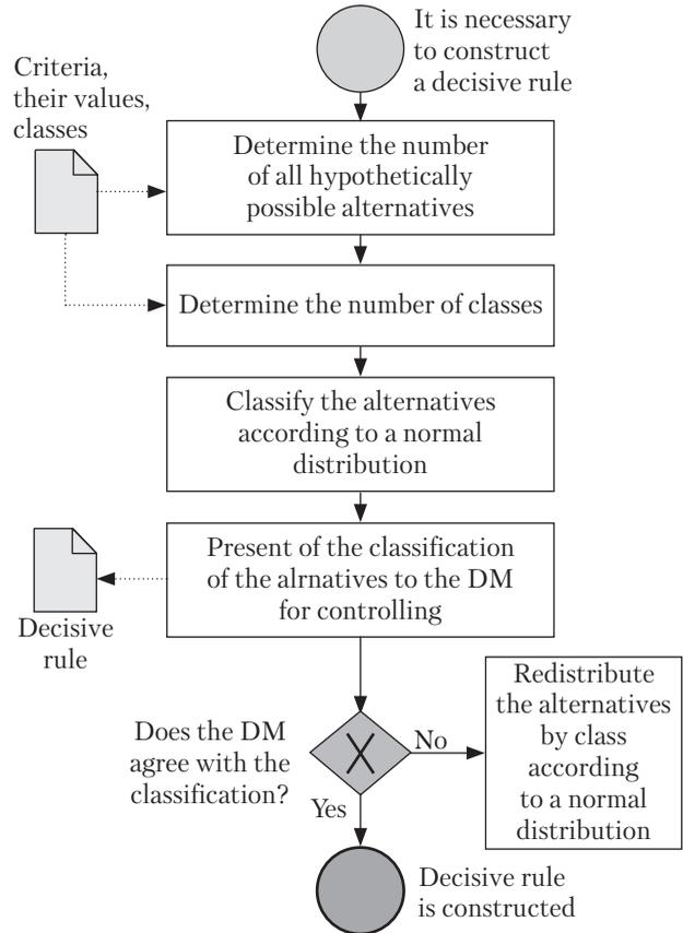
**Fig. 5.** Adapted procedure for building a decisive rule
