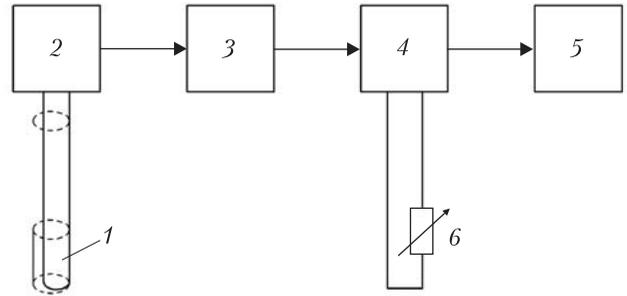
**Fig. 4.** Functional diagram of the capacitive level gauge of liquid helium: 1 – capacitive sensor; 2 – high frequency generator; 3 – frequency discriminator; 4 – DC amplifier; 5 – arrow indicator; 6 – resistor for setting “0”
