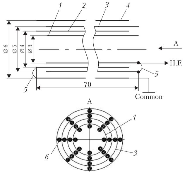
**Fig. 5.** Capacitive level sensor: 1, 2, 3, and 4 – metal tubes; 5 – wires; 6 – threads
