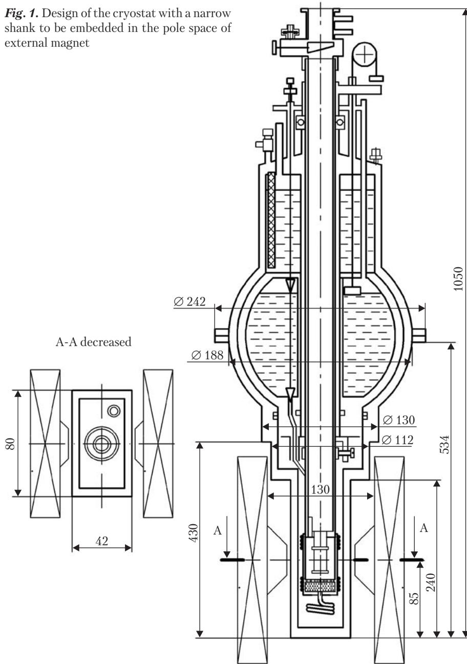
pouring liquid helium, placing a level gauge, and installing a needle valve for liquid helium supply, which is controlled by the handle.
