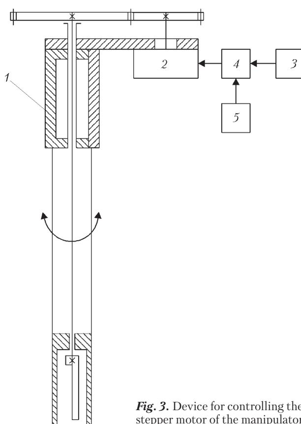
**Fig. 3.** Device for controlling the stepper motor of the manipulator
