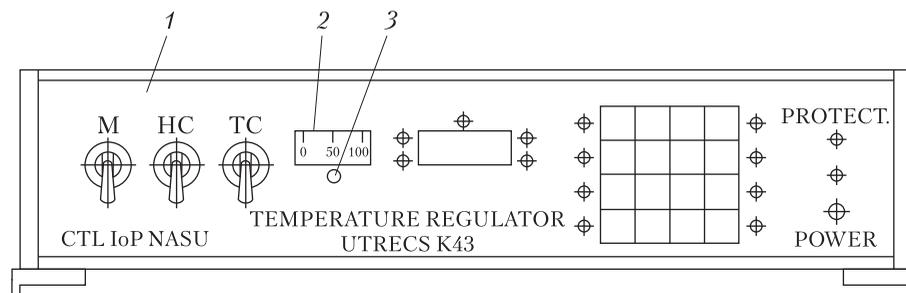
**Fig. 6.** Switch device of the capacitive indicator built in the temperature controller
