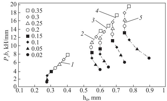
**Fig. 3.** Dependences  $P_{\text{CHM}}/b = \varphi(h_{\text{OHM}})$ , constructed from the results of modeling the parameters of cold rolling of 08kp steel strips ( $R = 300\text{ mm}$ ,  $f = 0.05$ ;  $q_0 = q_1 = 0$ ) with different degrees of preliminary work hardening: 1 –  $\varepsilon_{\text{ip}} = 0$ ; 2 –  $\varepsilon_{\text{ip}} = 0.4$ ; 3 – the same 0.5; 4 – the same 0.7; 5 – the same 0.9
