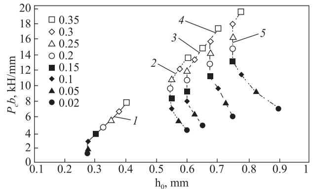
**Fig. 3.** Dependences  $P_{\text{CHM}}/b = \varphi(h_{\text{OHM}})$ , constructed from the results of modeling the parameters of cold rolling of 08kp steel strips ( $R = 300$  mm,  $f = 0.05$ ;  $q_0 = q_1 = 0$ ) with different degrees of preliminary work hardening: 1 –  $\epsilon_{ip} = 0$ ; 2 –  $\epsilon_{ip} = 0.4$ ; 3 – the same 0.5; 4 – the same 0.7; 5 – the same 0.9
