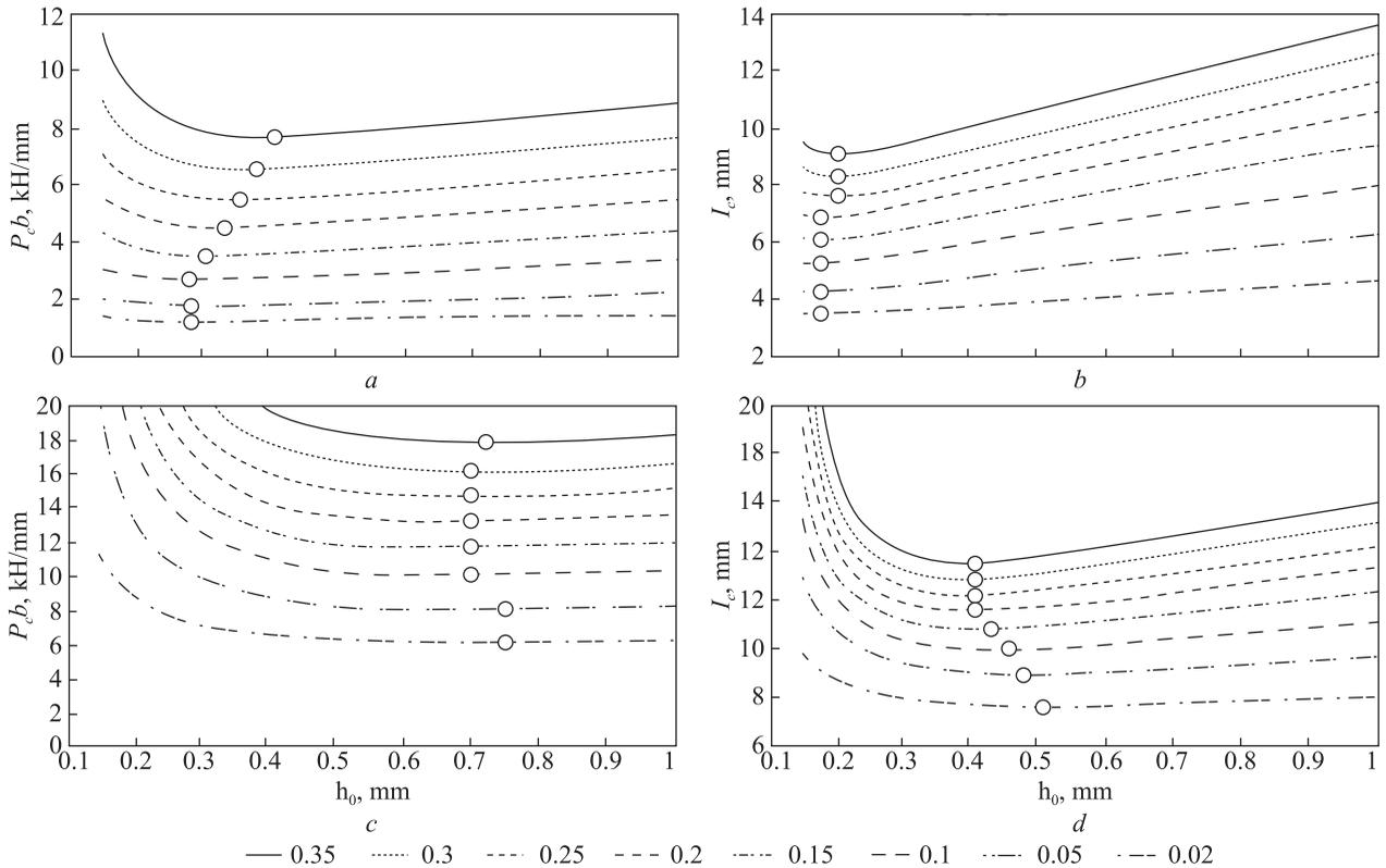
**Fig. 2.** Dependences  $P_c/b = \varphi(h_0)$  and  $l_c = \varphi(h_0)$ , constructed from the results of modeling the parameters of cold rolling of non-riveted ( $\epsilon_{np} = 0$ ) (a, b) and work-hardened ( $\epsilon_{np} = 0.75$ ) (c, d) strips made of 08kp steel ( $R = 300$  mm,  $f = 0.05$ ;  $q_0 = q_1 = 0$ )
