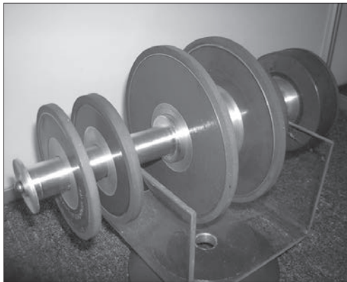
Fig. 7. Diamond abrasive wheel, shape 1A1
