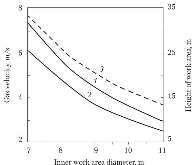
**Fig. 1.** Effect of work area diameter on gas velocity at the inlet (1), gas velocity at the outlet (2), and height of work area (3)
