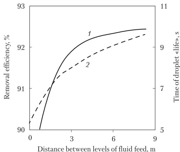
**Fig. 2.** Effect of distance between levels of fluid feed on effectiveness of reagent binding (1) and time of droplet «life» (2)
