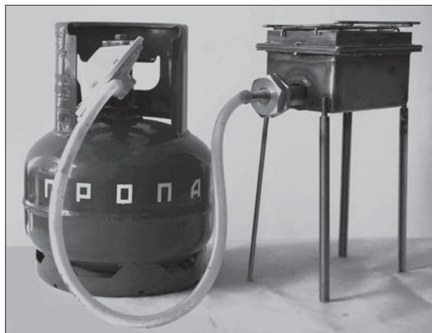
Fig. 5. Catalytic heat generator based on flameless combustion of methane or propane-butane mix
