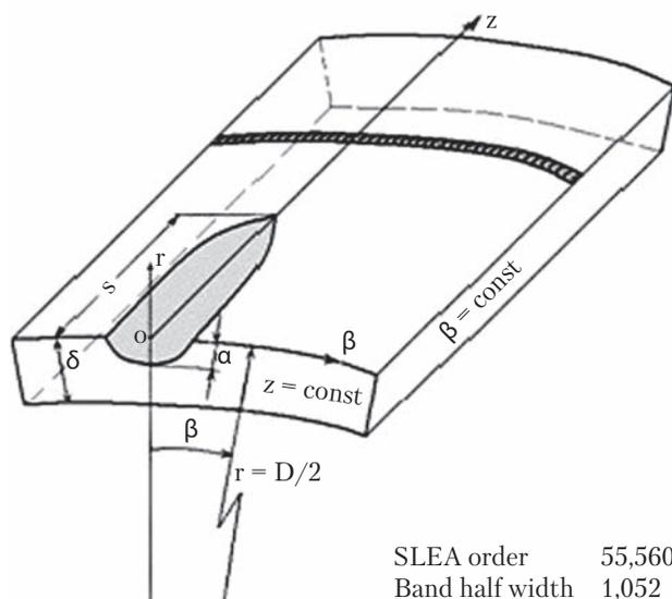
Fig. 7. Simulation of stress-strained state of weld structures in WeldPredictions\_g
