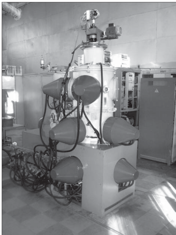
Fig. 1. General view of the facility consisting of three-modular vacuum chamber for deposition of cavitation-resistant coatings on turbine blades
