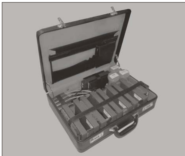
Fig. 11. General view of wireless AE diagnostic system
