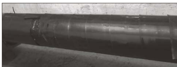
Fig. 3. 325 mm diameter pipe coated with BPC
