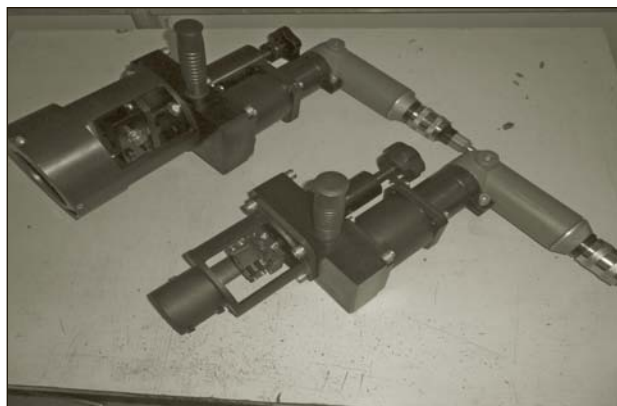
Fig. 8. General view of prototype end facers TRC38 U3.1 (right) and TRC76 U3.1 (left)
