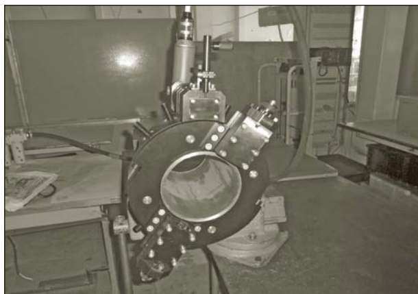
Fig. 9. General view of prototype cutter TTC660 U3.1
