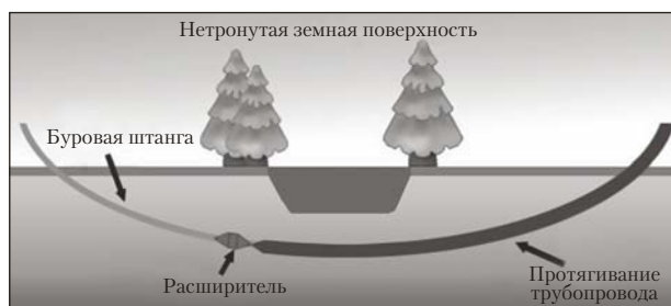
Fig. 6. Horizontal directed drilling
