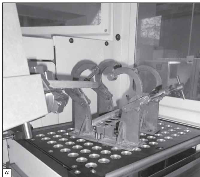
Fig. 5. Testing of software using Fanuc LR Mate 200 robot: a) mounting of a rib; b) assembled unit (rib)
