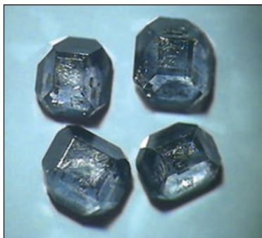
Fig. 4. General view of diamond single crystals of IIb type grown on crystal seed in the system Fe-Al-B-C (weight 2.0–2.5 ct)
