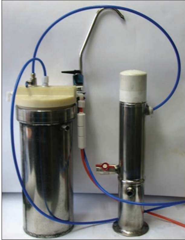
Fig. 3. Home installation with UV disinfection, capacity of 20–30 dm 3 /h, for purification of tap and brackish water
