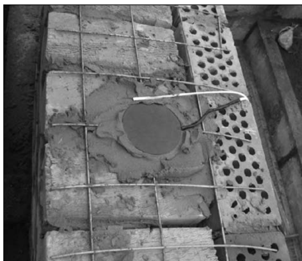
Fig. 5. Heat loss gauges mounted in the walling: 1 – rectangular heat flow transducer; 2 – round heat flow transducer with imbedded platinum resistance thermometers; 3 – copper resistance thermometer
