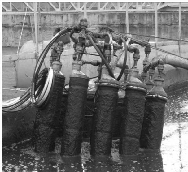
Fig. 6. Filter module brought up to the tank surface after operation without regeneration
