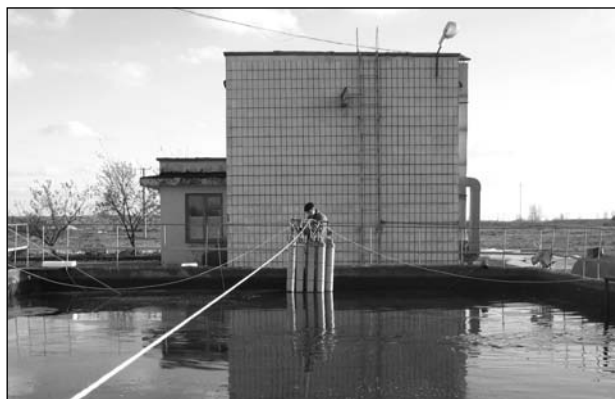
Fig. 4. Location of the pilot facility filter module in the tank to which aerobically stabilized treated sludge and supernatant water from draining beds are supplied
